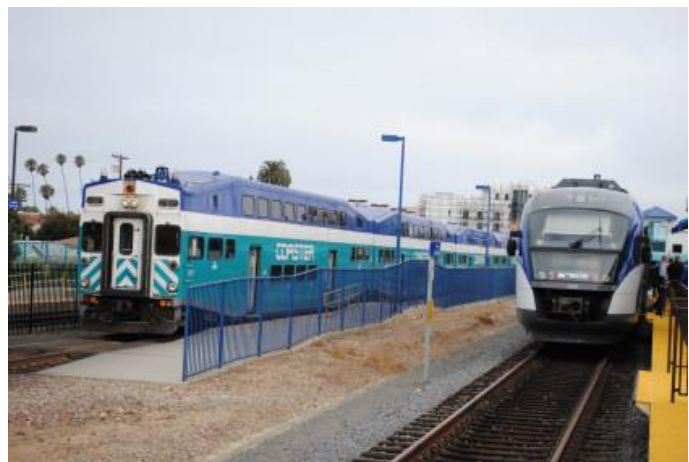
Figure 2: Coaster commuter rail (left) and Sprinter hybrid rail (right) share a station, but not tracks, at Oceanside, CA. Difference in size and design between the two modes is apparent. Source: http://www.trainweb.org/chris/13nps4.JPG
